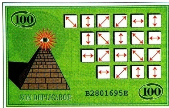
A quantum bank note, containing a secret set of polarized photons, cannot be copied by counterfeiters, who would disturb the photons by attempting to measure them.
